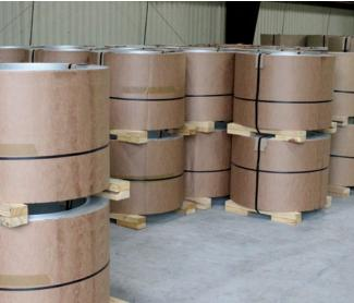
Berridge Manufacturing Company offers premium coated metal coil and flat sheet material in steel and aluminum. Its robust exterior durability, thanks to full-strength Kynar 500° or Hylar 5000° resins, makes it ideal for architectural projects demanding long-lasting, high-performance finishes.
