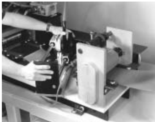
Fig. 1: The rollformer is outfitted with a swivel shear for making diagonal cuts.
